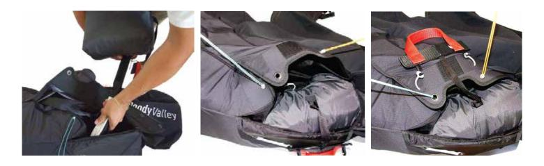
Thread a thin cord (such as paraglider riser cords) through each elastic loop. This will help close the pocket.
