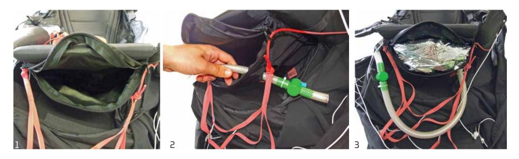
The ballast lodging is located beneath the seat. Open the zipper to access (1) the lodging, insert the discharge tube into the through-hole on the right (2) and install the ballast (3).
